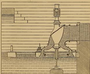
effect of the corresponding orifices, it follows that we cannot by means of this system of sluice reduce the volume of water so gradually as by means of the two independent valves mentioned above. These considerations led M. Girard to combine these two systems of sluices.
